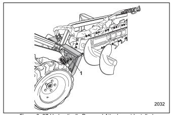
Figure 3–27 Hydraulically Powered Attachment Installed
